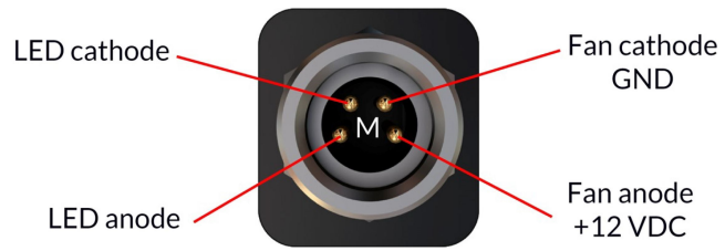
Figure 4.1: M8 Connector Pinout
