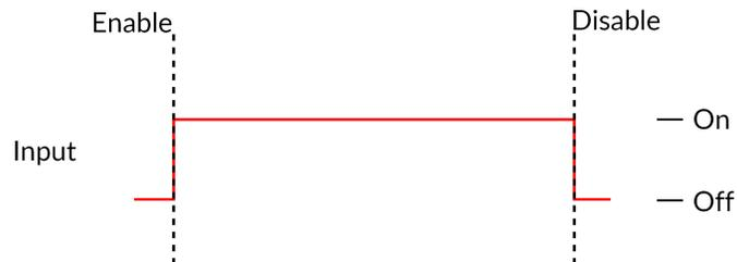
Figure 2.2: Constant Current Mode Driver Signal
