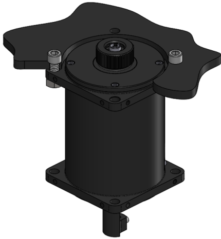
(a) Example of fixation with 6.8 mm holes
