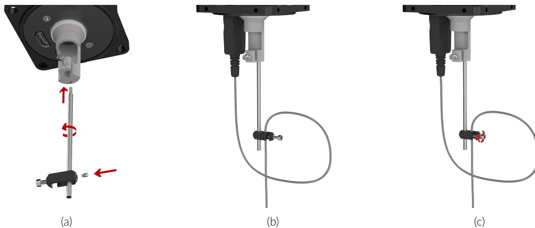
Figure 2.3: Rotary Joint Torque Rod and Loop Fixation
