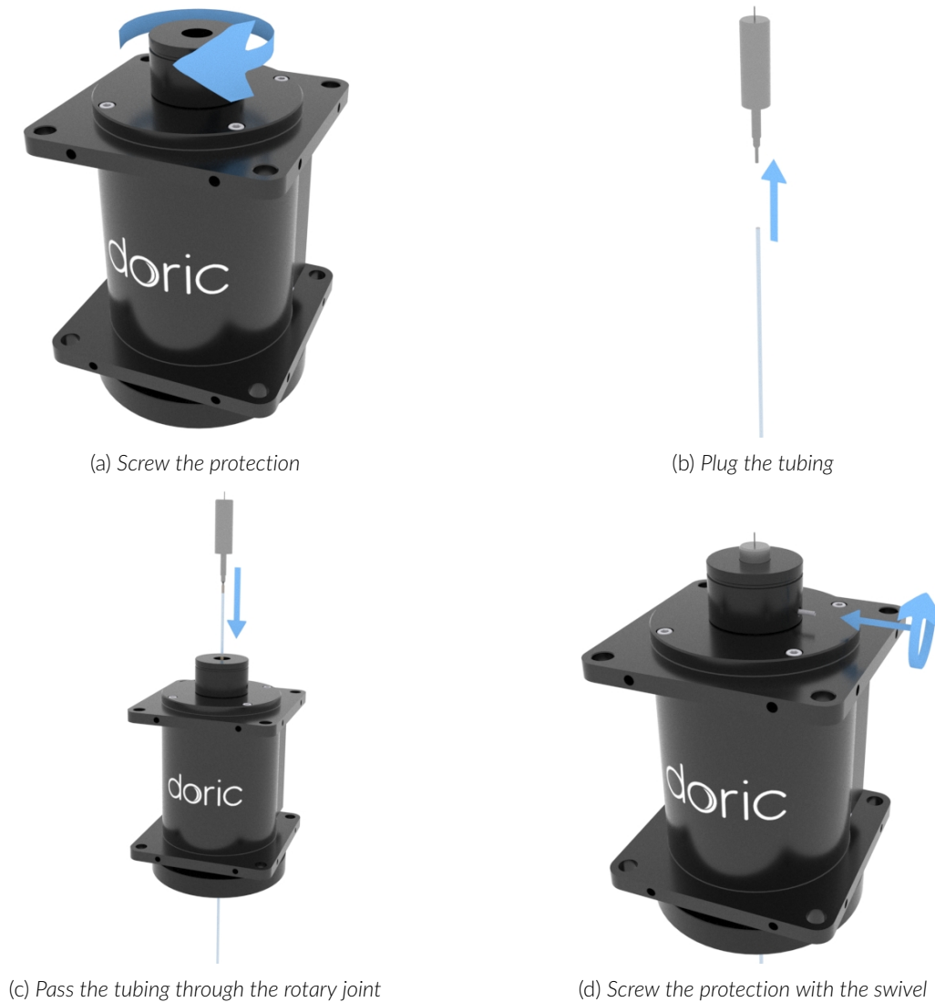
Figure 4.7: AHRJ-EL assisted rotary joint tubing installation
