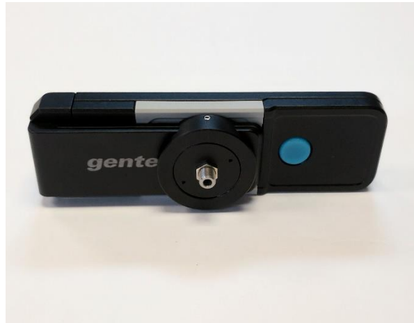
Figure 13 Proper way to store a PRONTO-Si with the threaded adaptor.
