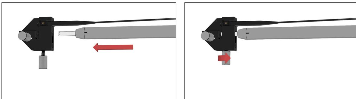
(a) Insert the opto-electric probe holder in the adapter
