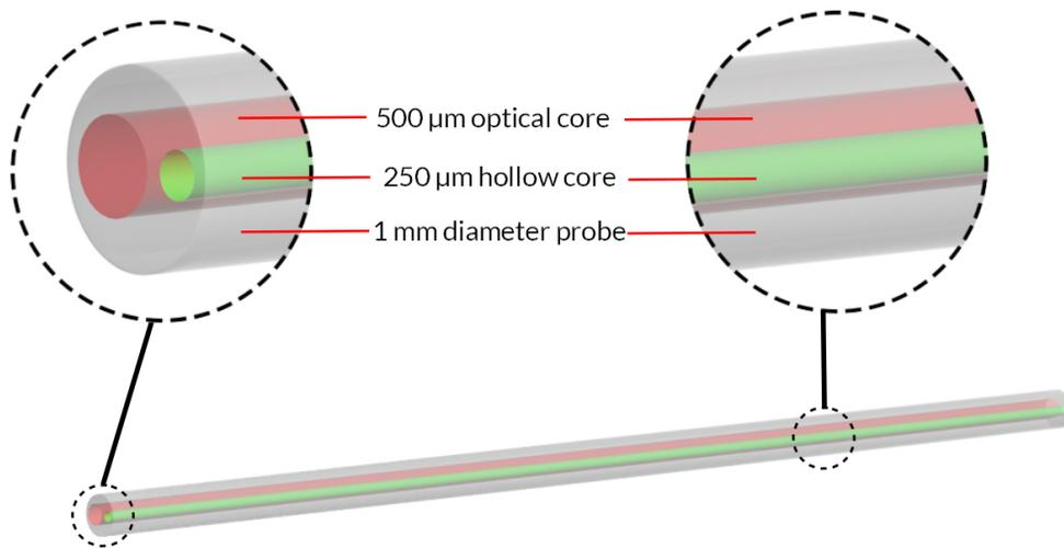
Figure 2.5: *Single-cell Opto-electric Probe-Raw Fiber*
