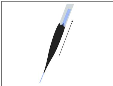
(c) Activate the pump to create negative pressure in the hollow-core fiber
