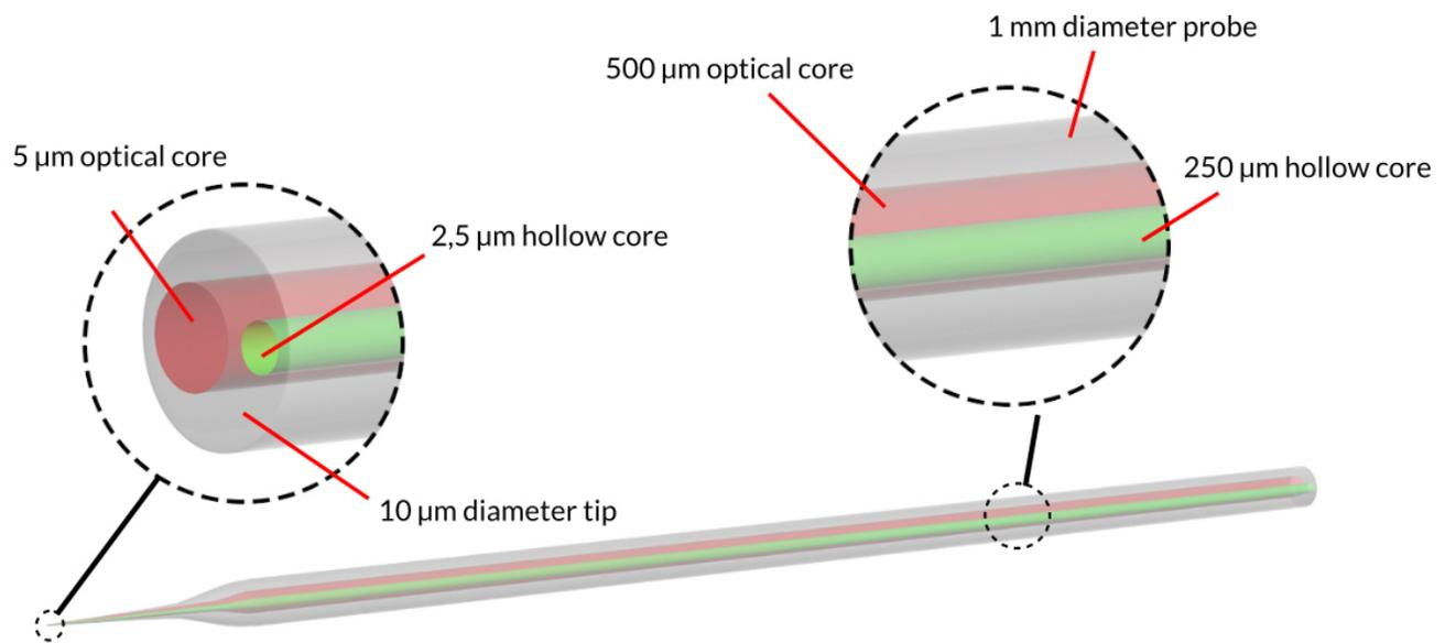
Figure 2.3: *Single-cell Opto-electric Probe Tips*; diameters indicated are typical values
