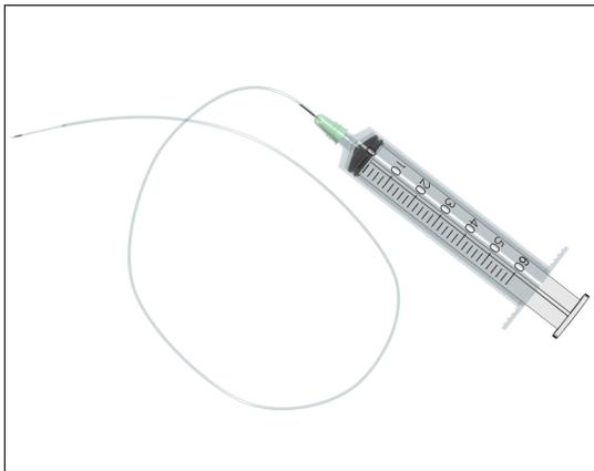
(a) Put a plastic tube at the tip of a large volume syringe and install the probe tip at the end
