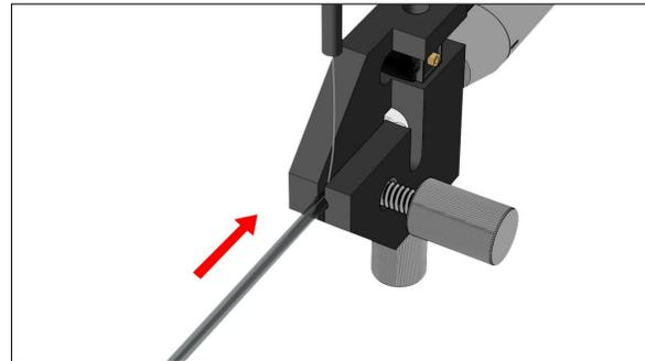
(f) Push the probe to create a contact with the zirconia ferrule
