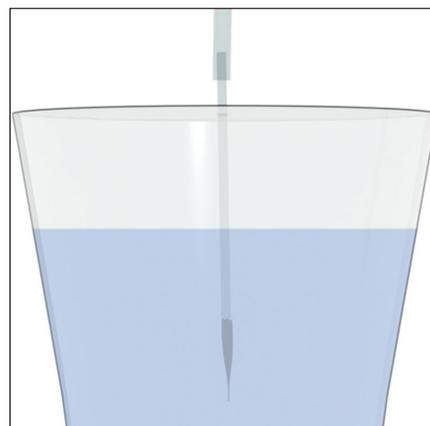
(b) Fill the syringe by pulling back the plunger
