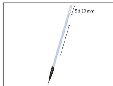
(d) Fill the hollow-core up to 5 to 10 mm from the large side
