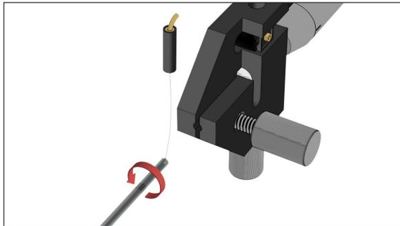
(e) Align the interconnect wire with the slot
