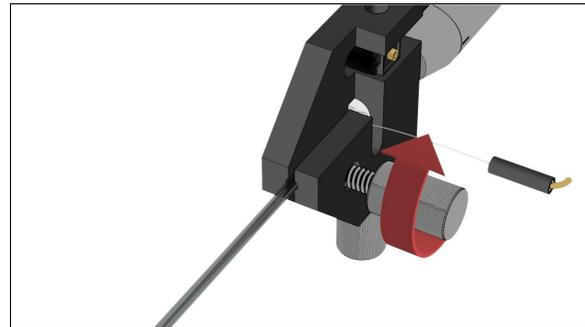
(h) Secure the probe tip position using the probe tip junction screw
