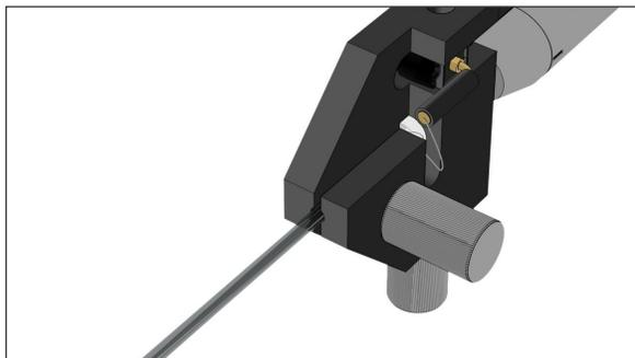
(i) Insert the gold metal end of the interconnect wire in the hole on the adapter
