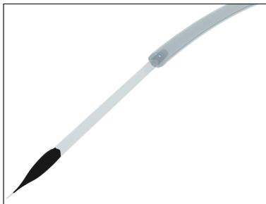
(a) Install the silicone tubing on the large end of the hollow-core fiber
