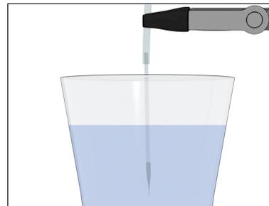
(b) Place the tapered tip of the probe in an electrolyte solution
