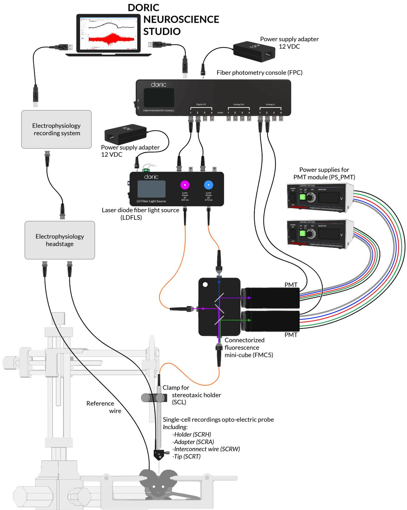
Figure 1.2: Single-cell Fiber Photometry and Electrophysiology System
