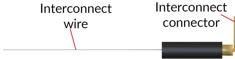
Figure 2.4: *Single-cell Opto-electric Interconnect Wire*
