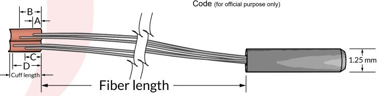
\*\*The schematic is an example of how the optical fibers can be set in the cuff.
