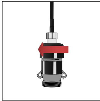
(a) Turn the barrel clockwise until you feel resistance then add 1/4 turn
