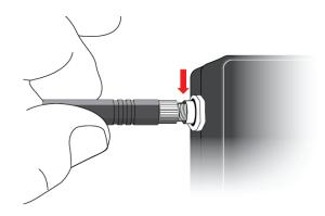
Turn clockwise the metal barrel of cable connector to tighten it.
