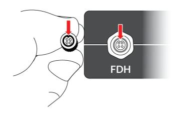
Make sure that the keys on both ends are aligned and gently insert the cable.
