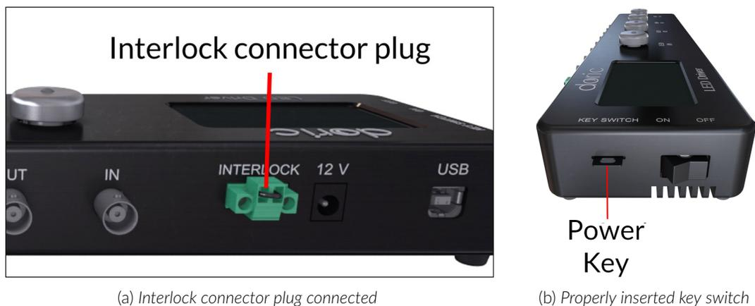
Figure 1.1: Safety procedure
