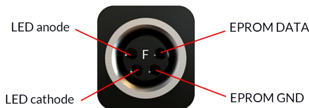
Figure 5.1: M8 Female Pinout (Microscope Driver)
