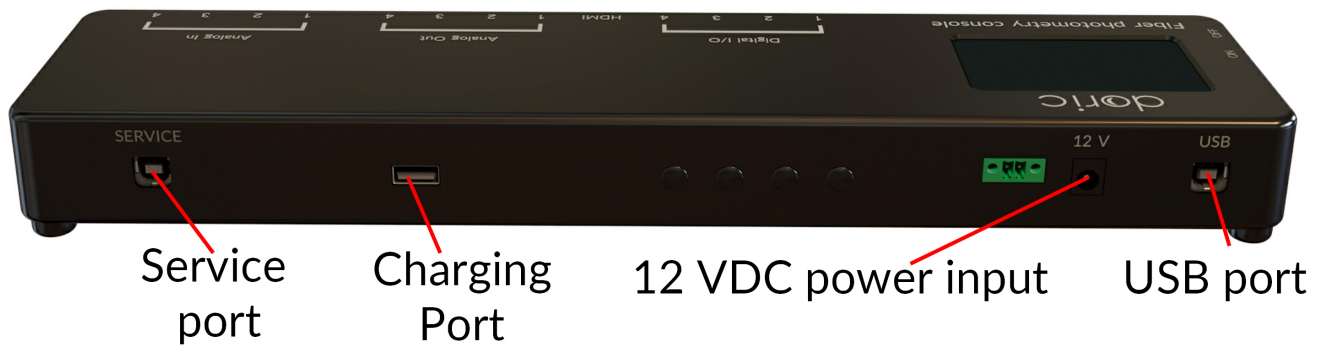
Figure 1.3: Back view: Maintenance and Power Supply
