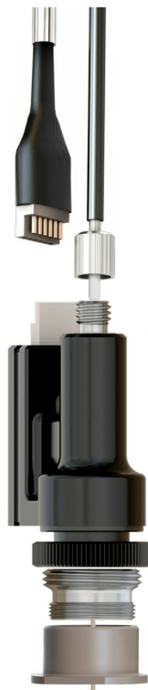
Figure 1.1: Miniature Fluorescence Microscopes In Exploded Format
