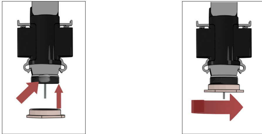
(a) Place glue drops into cannula thread
