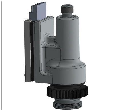
(a) Twist-on efocus Microscope body with protective cannula.
