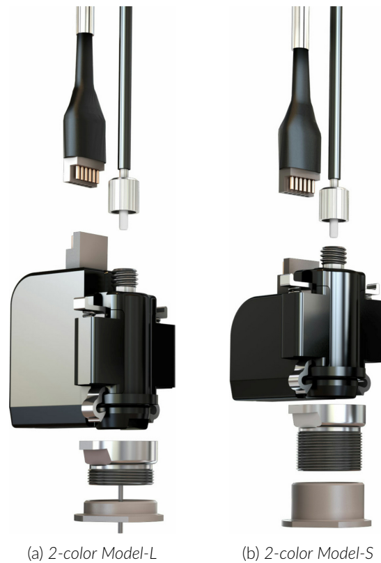
Figure 1.1: Miniature Fluorescence Microscopes In Exploded Format
